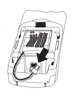
Place the battery pack inside the battery compartment, and slide the battery cover back on.
